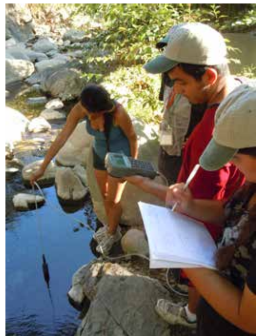
At Wheeler Creek on Los Padres Forest; students use the 9828 Multiparameter water quality portable meter, a professional-grade device that tests/analyzes to the highest specifications up to 13 parameters of water.
