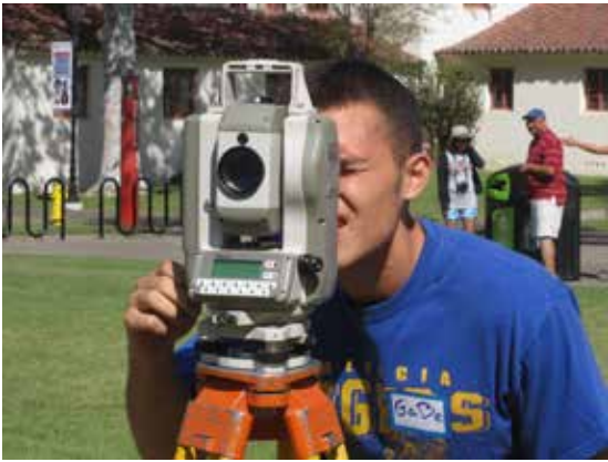
The Robotic field station uses laser beams and digital equipment to input various data to generate topographical maps and more for precise land surveys.
